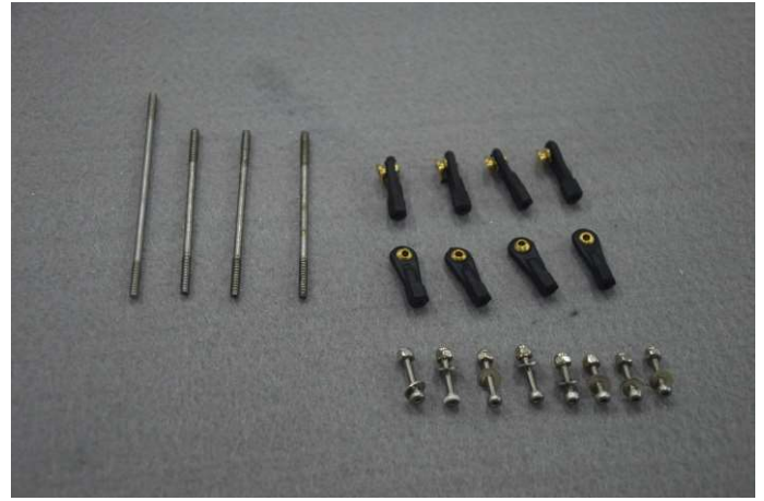
24.推杆安装,注意最长尺寸为升降用推杆.
